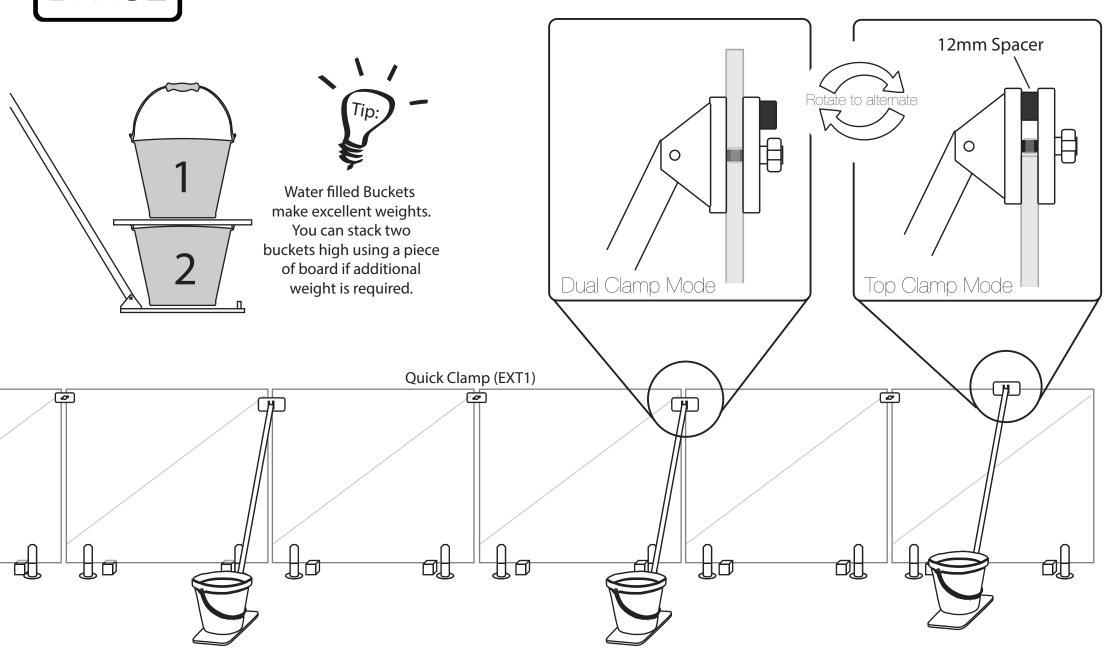
In low wind situations, use QuickClamps to reduce the number of EzyBrace required:
