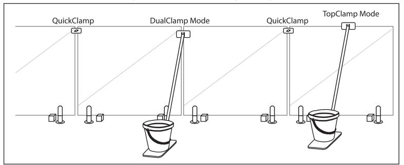
For strongest bracing, do not use QuickClamps & finish each run using TopClamp mode:
